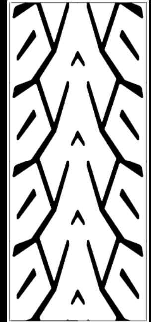
Grooved side profile (cornering / grip)
